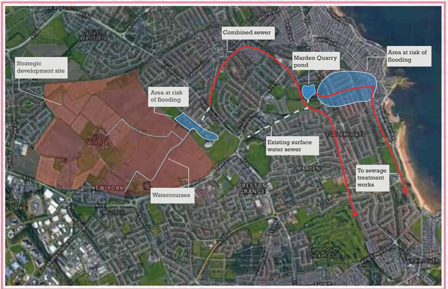
Figure 2: Pre Project Drainage Arrangement
