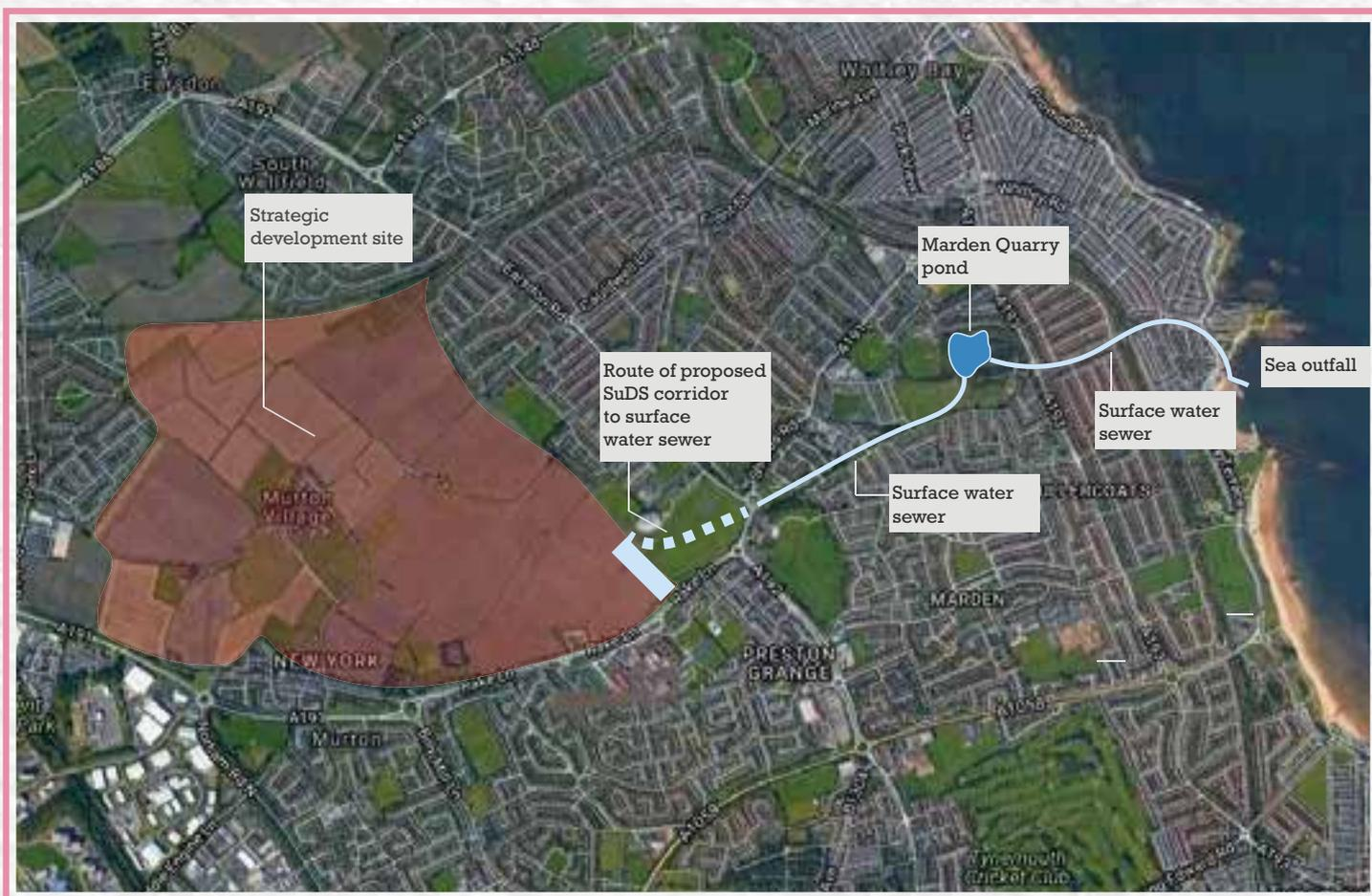
Figure 3: Post Project Drainage Arrangement
