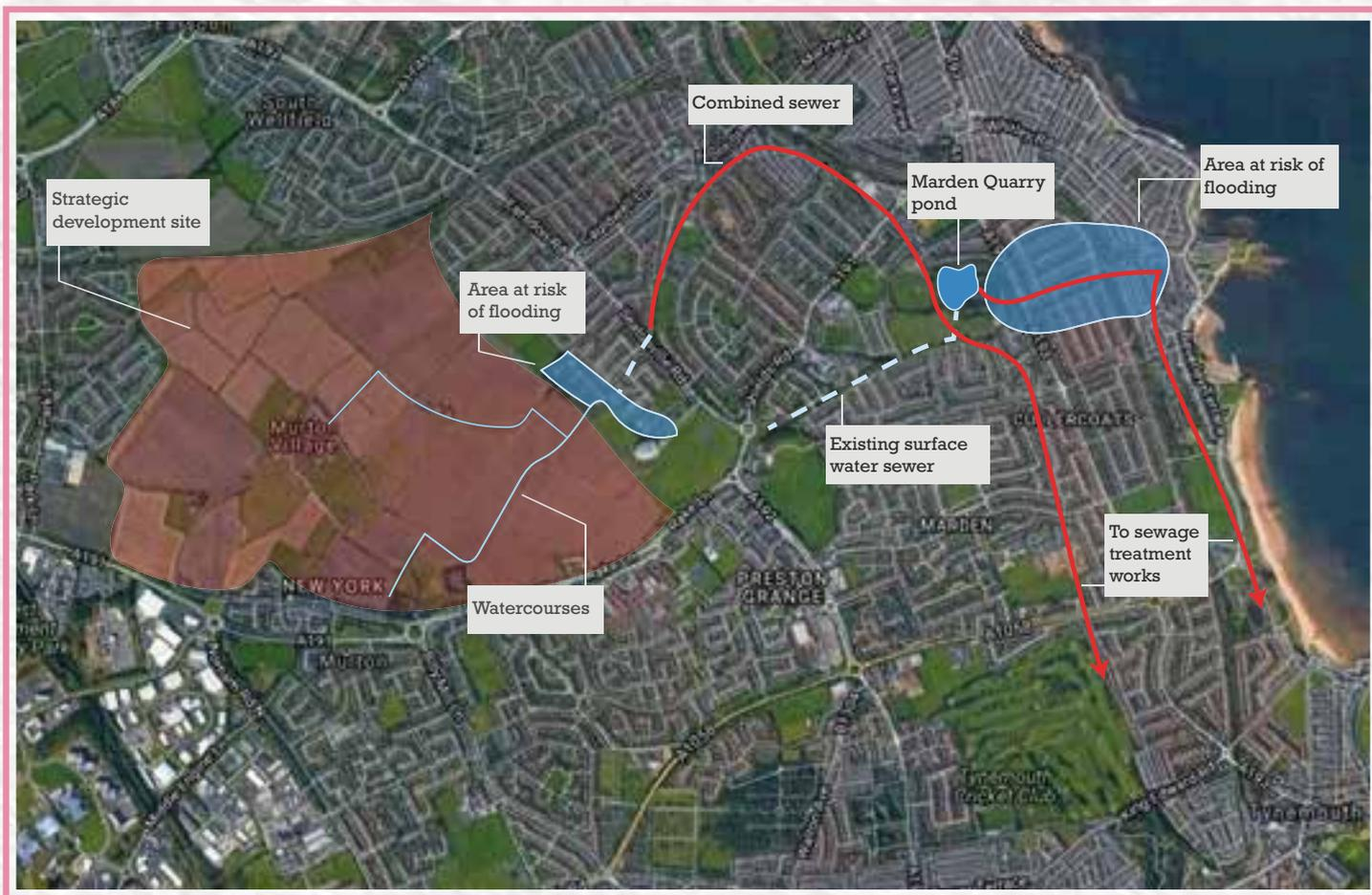
Figure 2: Pre Project Drainage Arrangement
