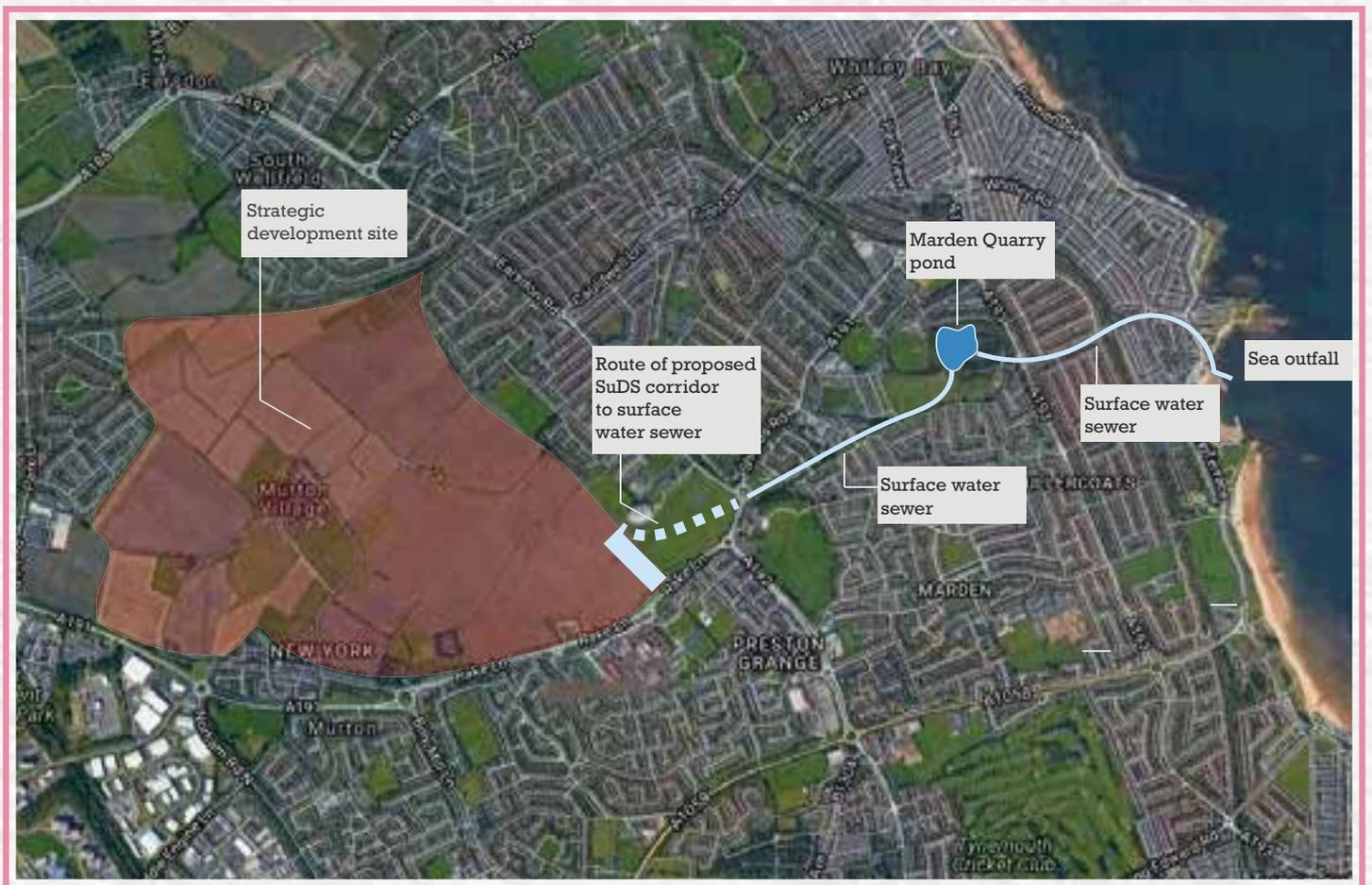
Figure 3: Post Project Drainage Arrangement
