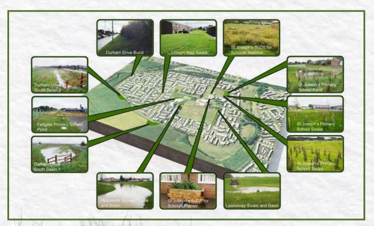
Figure 3: Schematic of SuDS elements
