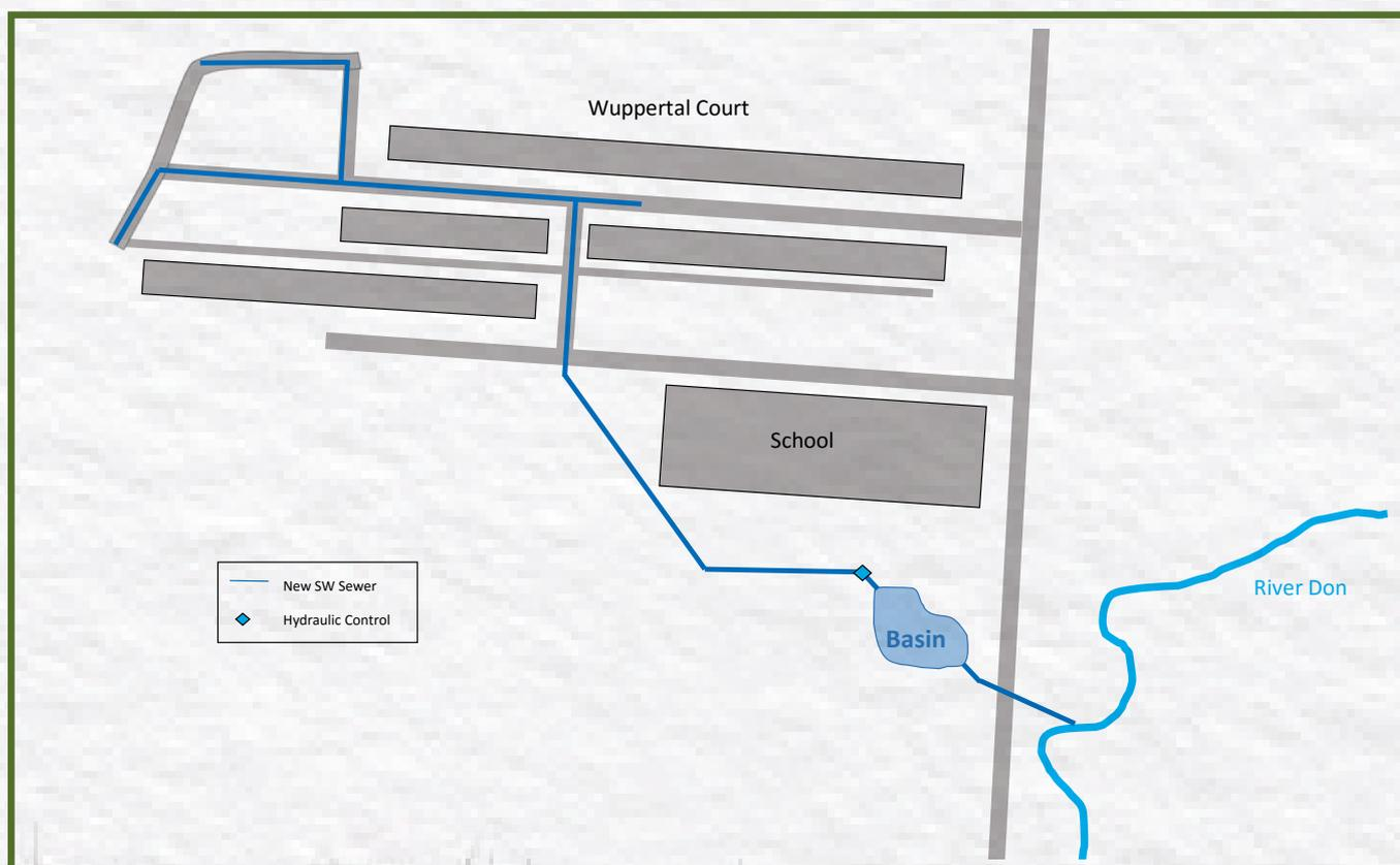
Figure 3. Schematic of surface water elements
