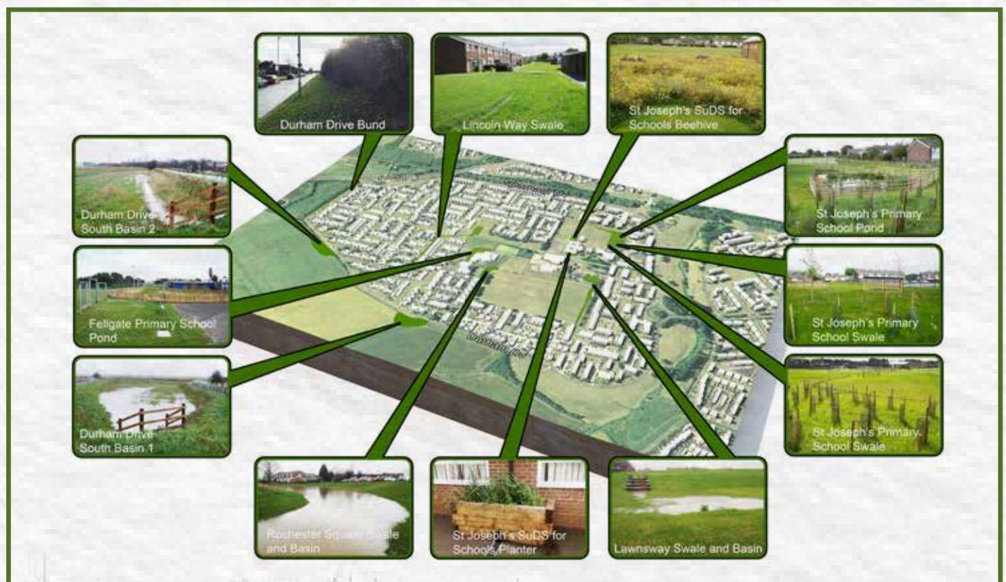
Figure 3: Schematic of SuDS elements
